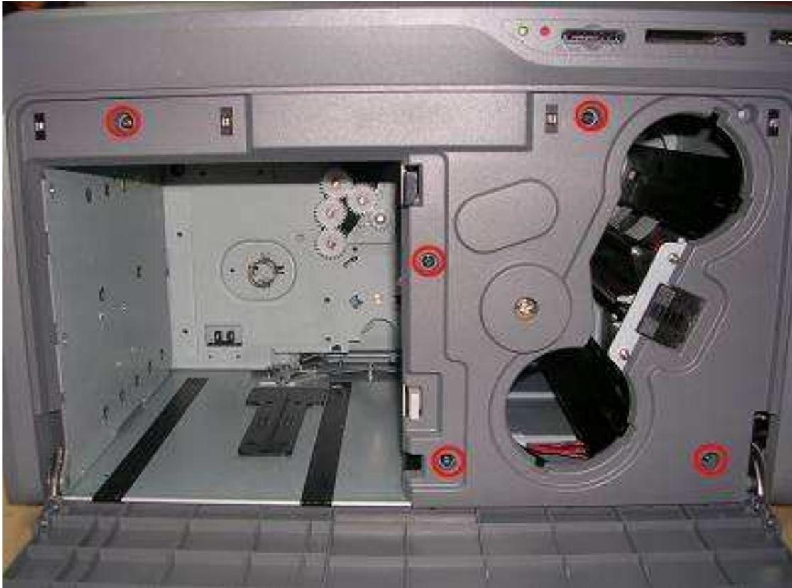
[Step 2] Turn the printer around to the bottom; you'll see that there are total 13 screws shown as below picture. Remove 2 screws of right, and then can take off the right cover (CASE\_RIGHT\_A5RT). Remove 6 screws both front/back sides, and then take out front cover (CASE\_FRONT\_A5RT) and (CASE\_BACK\_A5RT). Remove 5 screws of left that hold (CASE\_LEFT\_A5RT).
