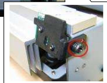
[Step 4] Replace the new ribbon LED/sensor and assemble it in the reverse order of the disassembly procedure.
