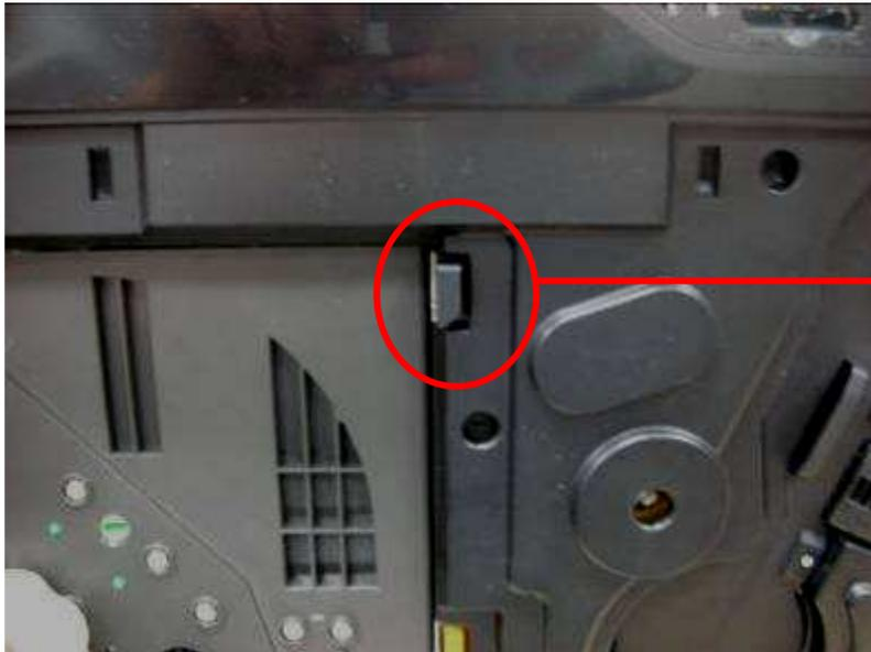
Any adjustment that needs disassembly of appearance cover, the door sensor is required to be enabled (pressed-in) in order to have the printer is ready mode.
