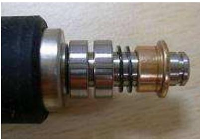
Note: Please noticed the related position between the bearing, washer and oil-retaining bearing.
