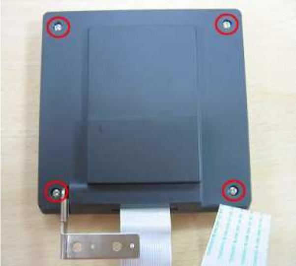
[Step 5] Replace the new LCD\_BD and assemble it in the reverse order of the disassembly procedure.
