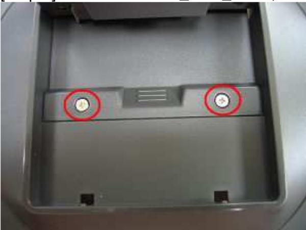
[Step 4] Remove 4 screws that hold LCD panel frame cover, and then take off the LCD\_BD.
