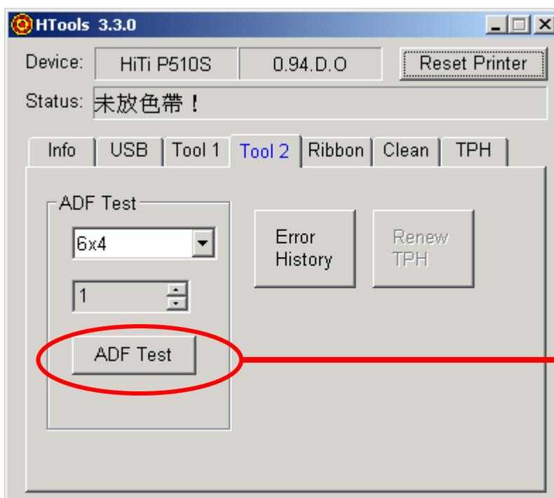
Press this single test button to start the paper feeding function.
