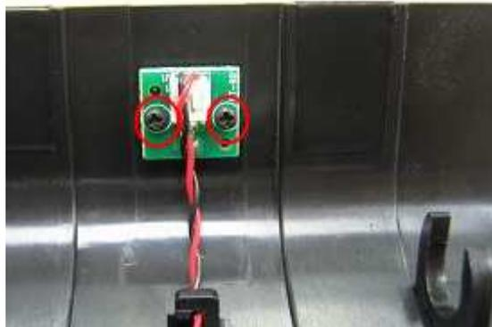
[Step 3] Replace the new Jam Sensor and assemble it in the reverse order of the disassembly procedure.
