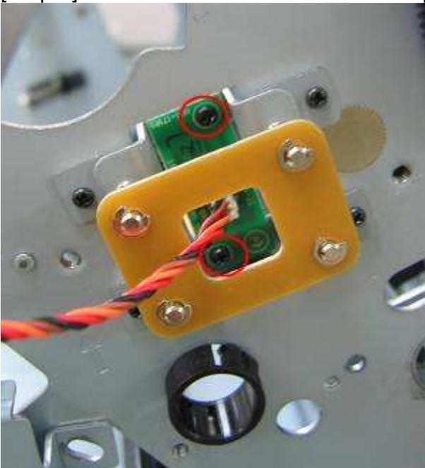
[Step 3] Replace the new IC chip sensor and assemble it in the reverse order of the disassembly procedure.
