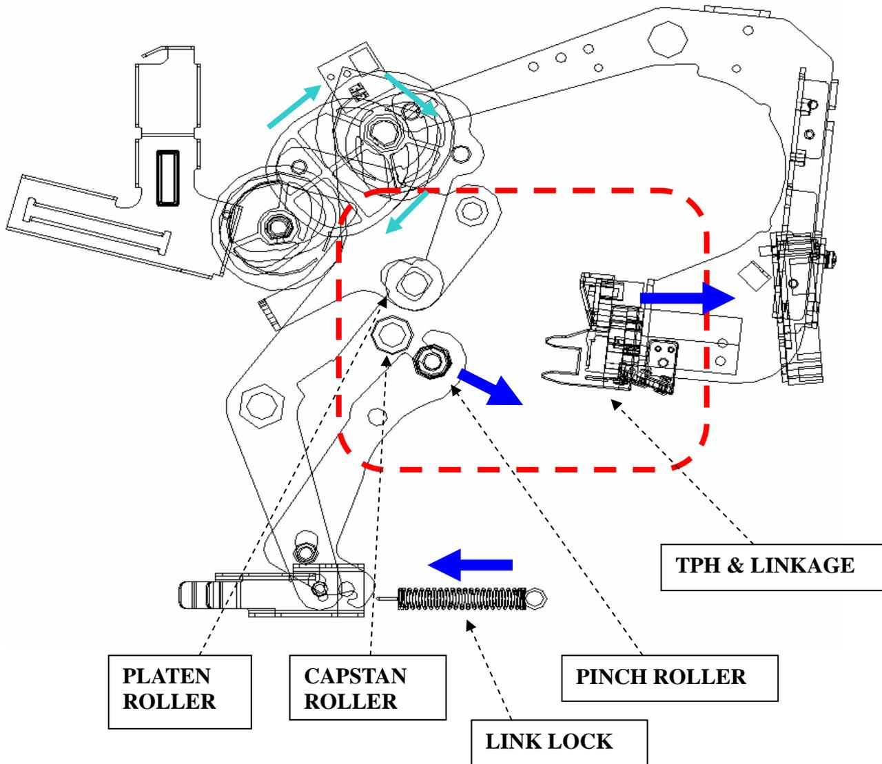
**● Cam Motion – Load****Q1(cam platen position)**
