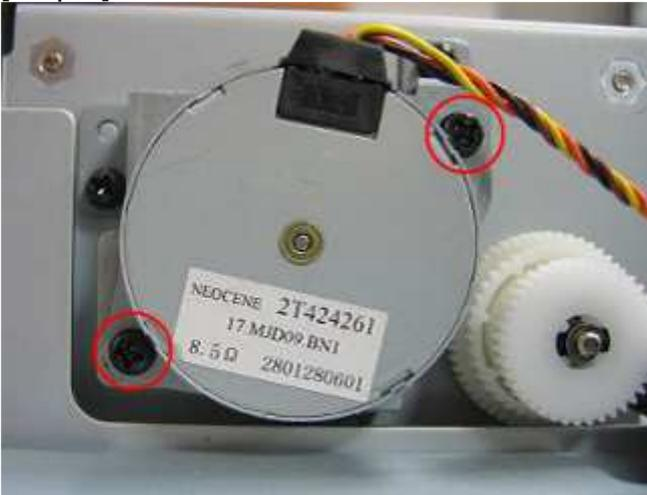
[Step 3] Replace the new cutter door motor and assemble it in the reverse order of the disassembly procedure.
