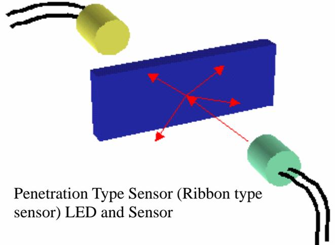
Penetration Type Sensor (Ribbon type sensor) LED and Sensor
