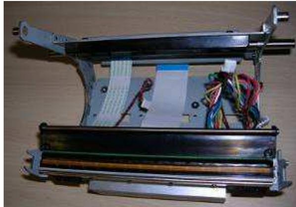
[Step 1] Remove "DOOR\_RIGHT\_A5RT", "CASE\_RIGHT\_A5RT", "CASE\_LEFT\_A5RT", "CASE\_BACK\_A5RT" "CASE\_TOP\_A5RT", "MAIN\_BD" and "RIBBON REVERSE\_MOTOR\_FRAME" according to [Procedure No. 1, 2, 3 and 9](#)
