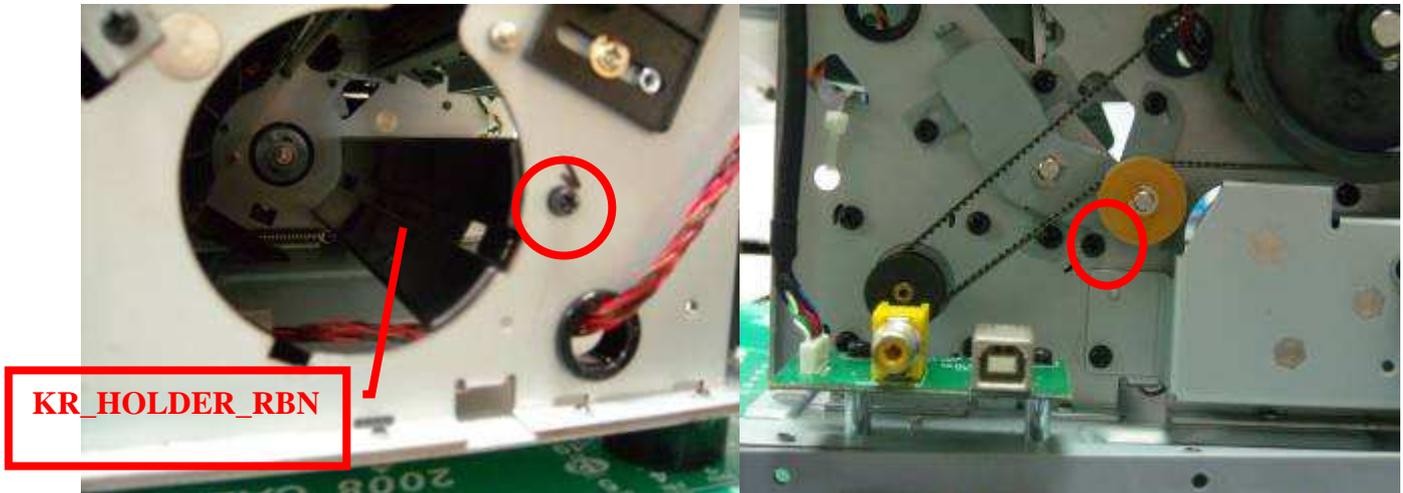
[Step 3] Unplug 3 connectors and remove 4 screws that hold FAN ASSY
