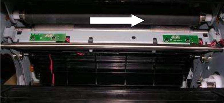
[Step 6] Replace the new CAPSTAN\_ROLLER\_A5 and assemble it in the reverse order of the disassembly procedure.
