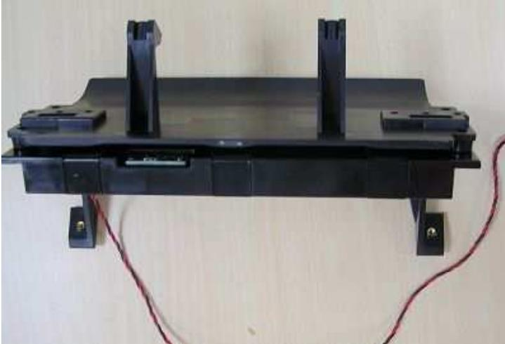
[Step 1] Remove "DOOR\_RIGHT\_A5RT", "CASET\_RIGHT\_A5RT", "CASE\_LEFT\_A5RT", "CASET\_FRONT\_A5RT" "CASE\_BACK\_A5RT" "CASE\_TOP\_A5RT", "MAIN\_BD", "ROLLER\_EXIT\_PINCH\_CUTTER\_A5", "TRAY\_EXIT\_ASSY", "RIBBON REVERSE MOTOR\_FRAME" "TPH Linkage", "CAPSTAN\_ROLLER\_A5", "ROLLER\_PLATEN\_NEW\_A5" and "ROLLER\_PINCH\_A5" according to [Procedure No. 1, 2, 3, 9, 14, 16, 17, 19, 20 and 21](#)
