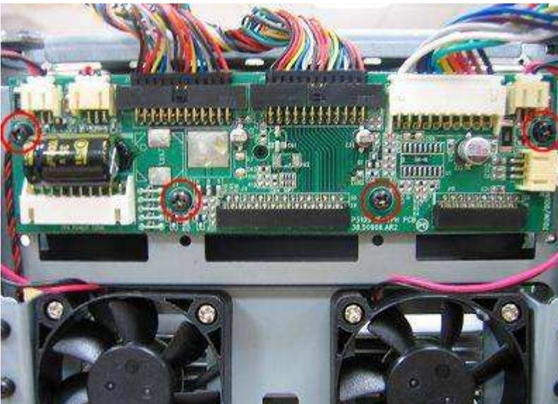
[Step 3] Replace the new TPH\_BD and assemble it in the reverse order of the disassembly procedure.
