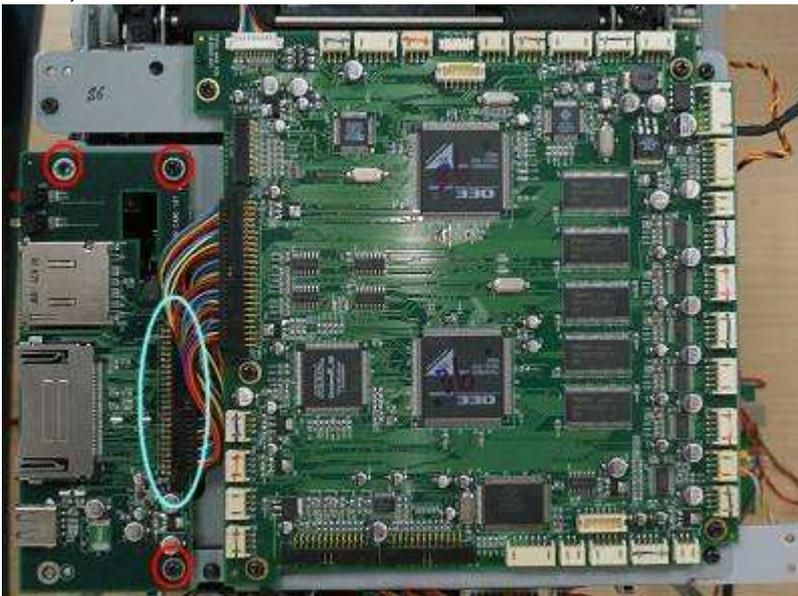
[Step 3] Replace the new CARD\_BD and assemble it in the reverse order of the disassembly procedure.
