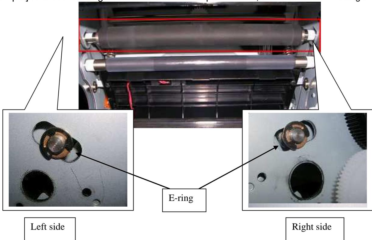
[Step 3] Remove 2 clamps from both sides of the platen roller, slide the roller to the right, and then pull it out to the front. Remove the oil-retaining bearing together. (The oil-retaining bearing is used to install the platen roller.)
