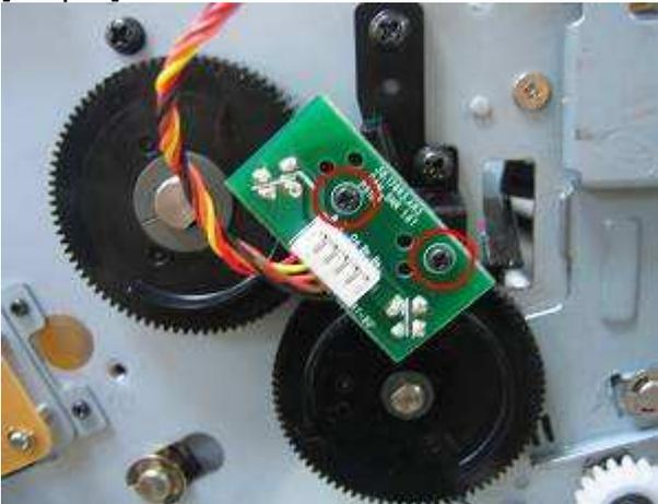
[Step 3] Replace the new cam sensors and assemble it in the reverse order of the disassembly procedure.
