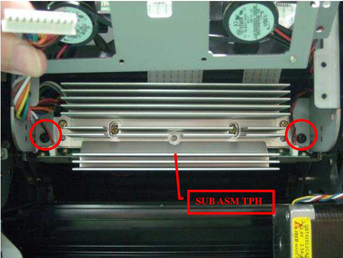
[Step 4] Remove 3 screws that hold TPH ASSY and then take off TPH ASSY.
