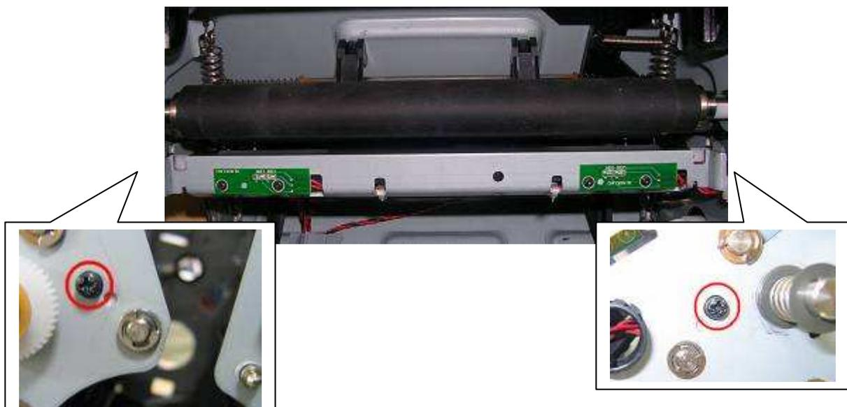
[Step 4] Remove 2 clamps from both sides of the pinch roller, slide the roller to the right, and then pull it out to the front. Remove the oil-retaining bearing together.
