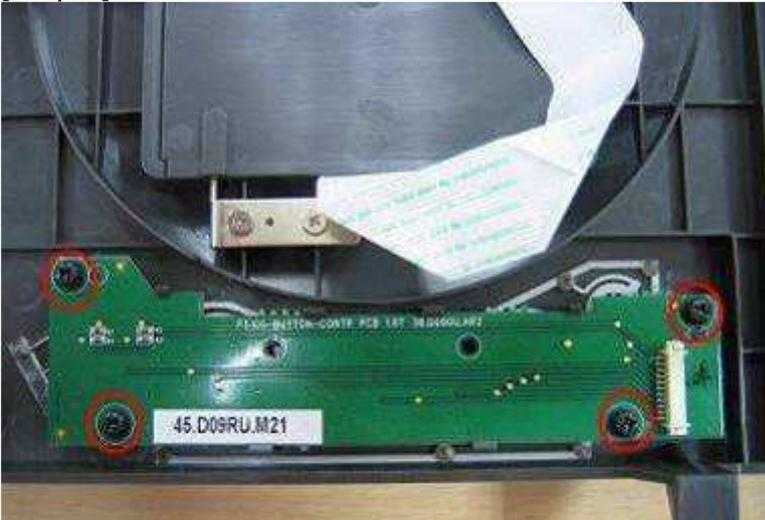
[Step 3] Release clutches that hold the BUTTON\_BD, and then take off the BUTTON\_BD.
