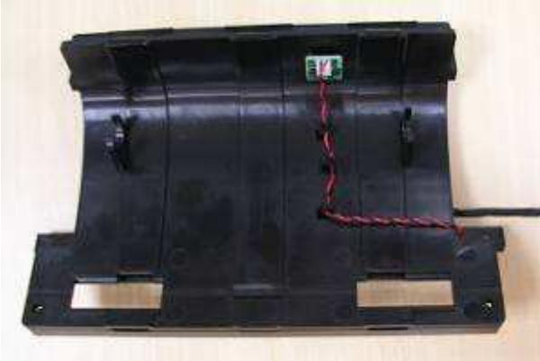
[Step 1] Remove "DOOR\_RIGHT\_A5RT","CASET\_RIGHT\_A5RT","CASE\_LEFT\_A5RT", "CASE\_BACK\_A5RT" "CASE\_TOP\_A5RT","MAIN\_BD" and "ROLLER\_EXIT\_PINCH\_CUTTER\_A5" according to [Procedure No. 1, 2 ,3 and 14](#)
