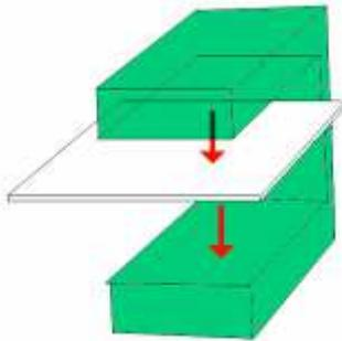
Penetration Type Sensor (Jam type sensor)
