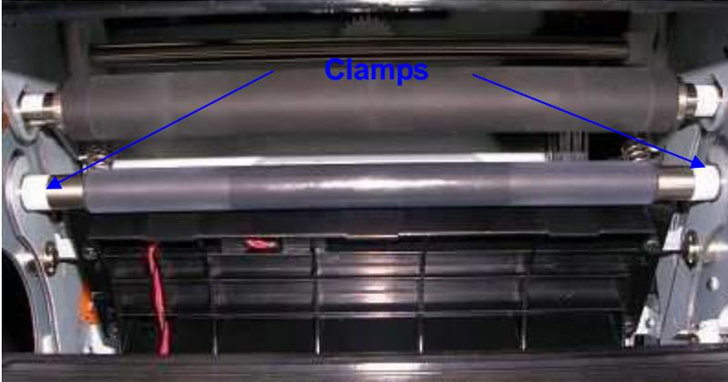
[Step 5] Replace the new pinch roller and assemble it in the reverse order of the disassembly procedure.
