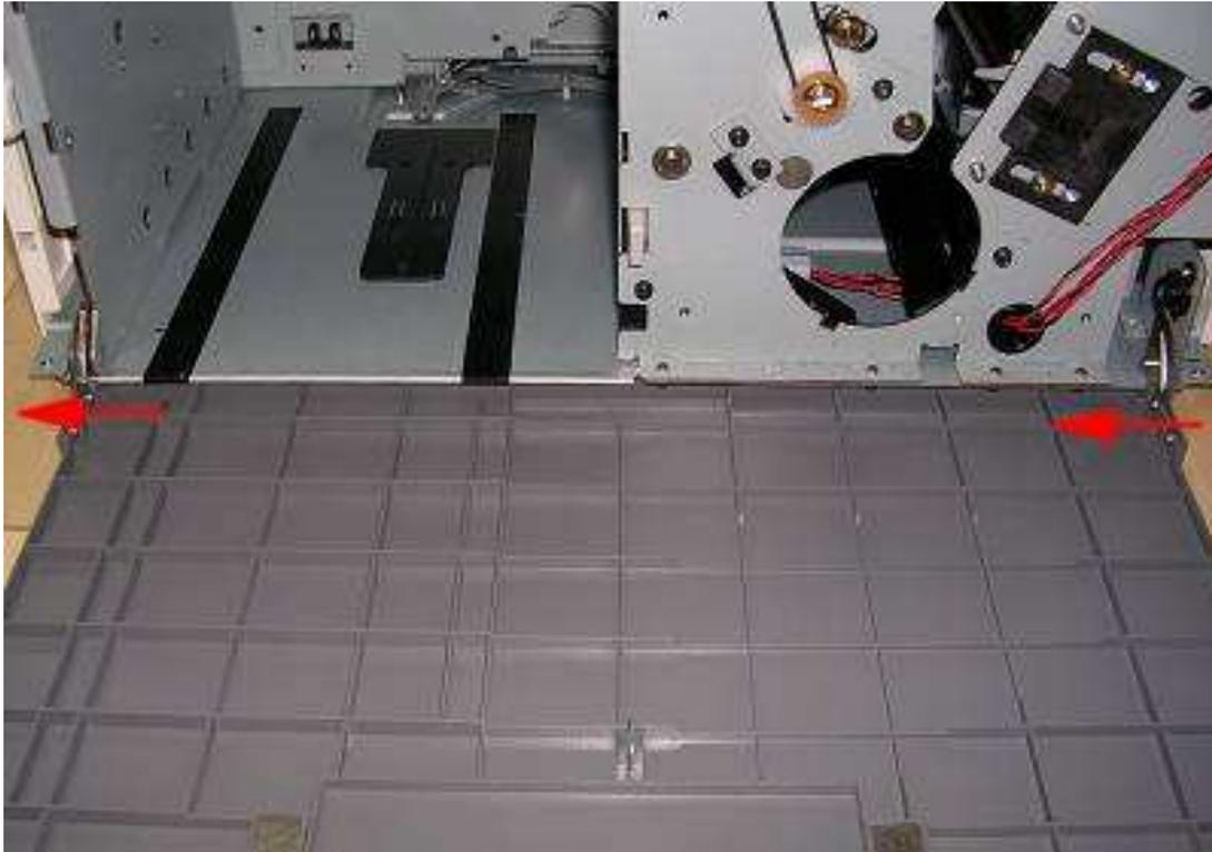
[Step 4] Now turn the printer to left side, remove 3 screws that hold CASE\_LEFT\_A5RT, then take off CASE\_LEFT\_A5RT.
