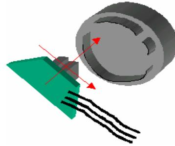
Penetration Type Sensor (Cam Sensor Type)
