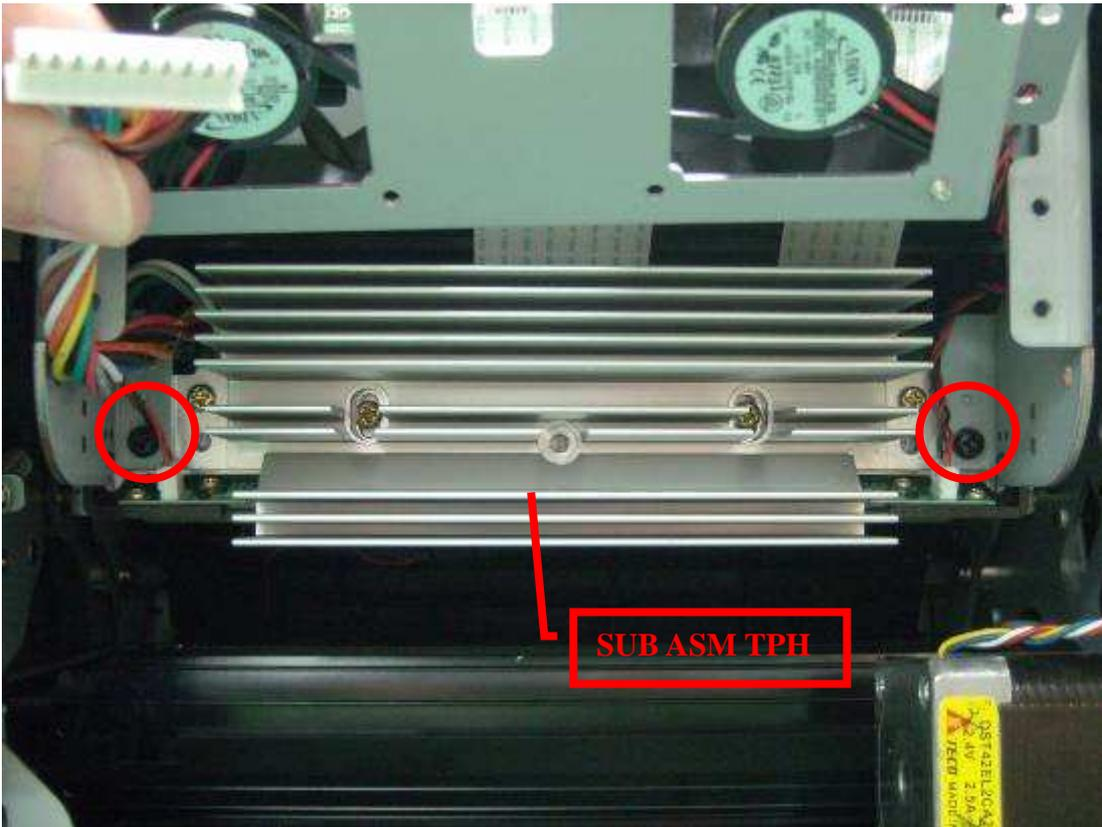
[Step 5] Remove 3 screws that hold TPH ASSY and then take off TPH ASSY.
