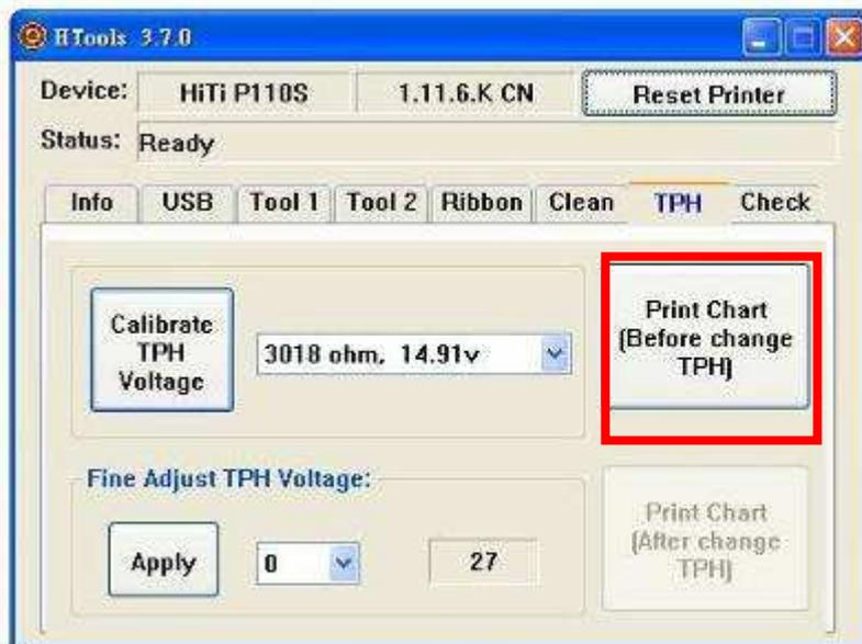
2. According to new TPH  $\Omega$ , choose the close TPH  $\Omega$  and Voltage.
