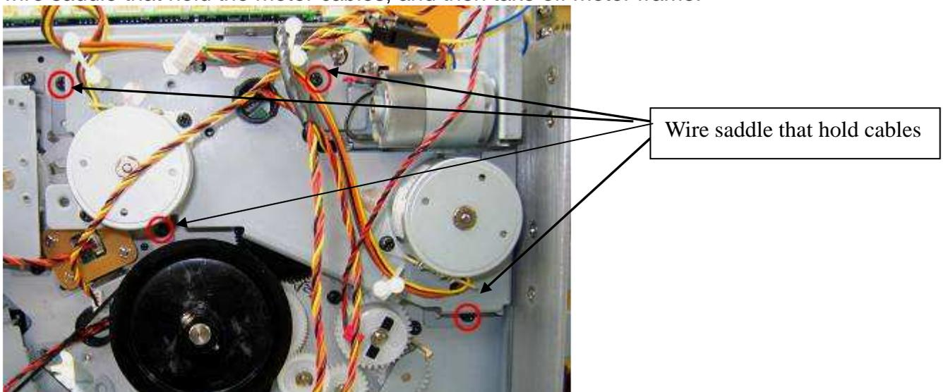
[Step 3] Replace the new cam pinch & cam platen motor frame and assemble it in the reverse order of the disassembly procedure.
