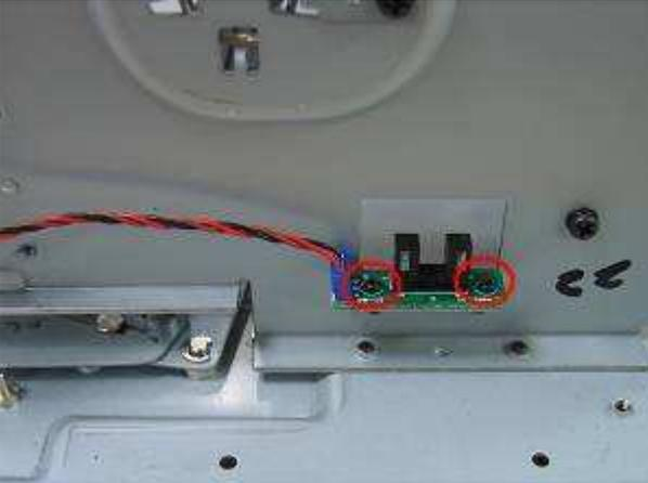
[Step 5] Replace the new paper box sensor and assemble it in the reverse order of the disassembly procedure.
