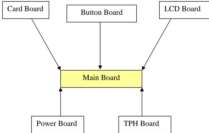
**Notes:** All boards are connected to the main board, so in most cases, during problem checking, we advise to start with the individual boards before checking the main board.
