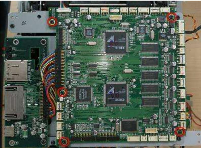
[Step 3] Replace the new MAIN\_BD and assemble it in the reverse order of the disassembly procedure.
