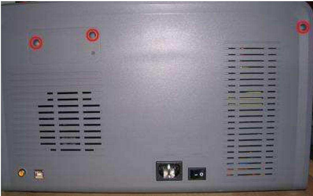
[Step 5] Remove 2 connectors that connect with power core and POWER BD, remove 1 screw that ground, and then take off CASE\_LEFT\_A5RT.
