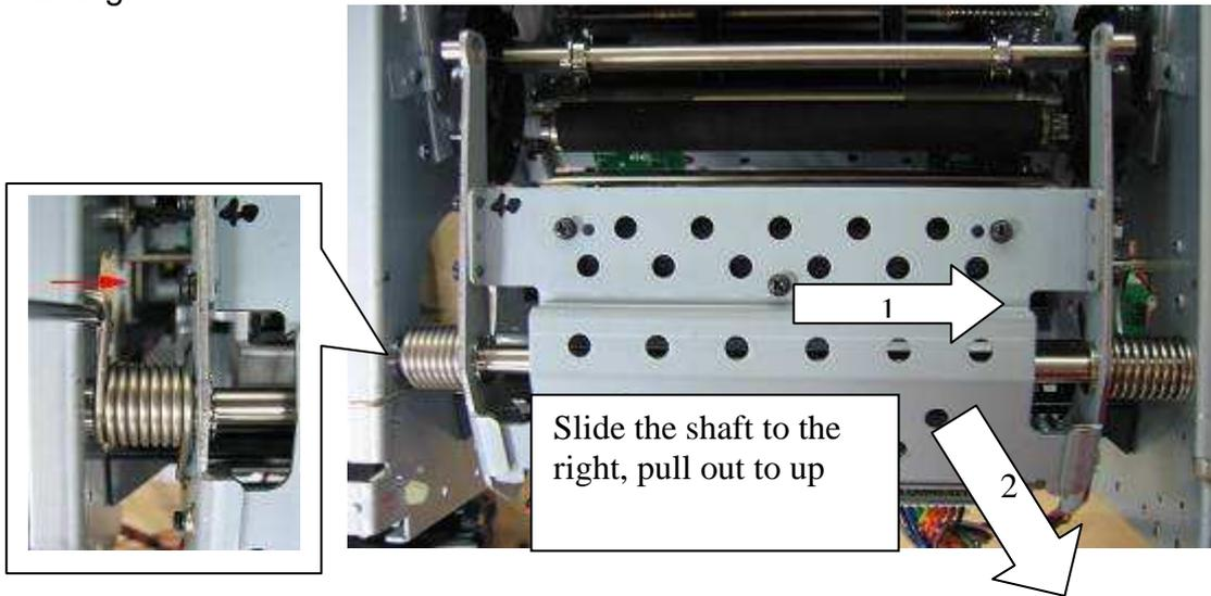
[Step 4] Replace the new TPH linkage and assemble it in the reverse order of the disassembly procedure.
