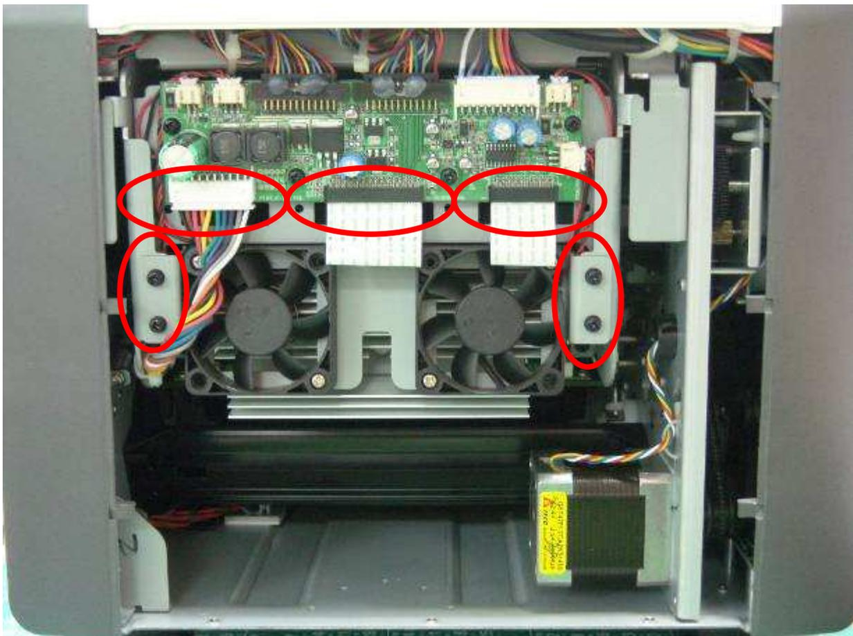
[Step 4] Remove 2 screws that hold SUB ASM TPH A5RT, and then take off SUB ASM TPH A5RT
