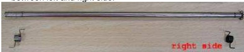
[Step 4] Replace the new ROLLER\_EXIT\_PINCH\_CUTTER\_A5 and assemble it in the reverse order of the disassembly procedure.
