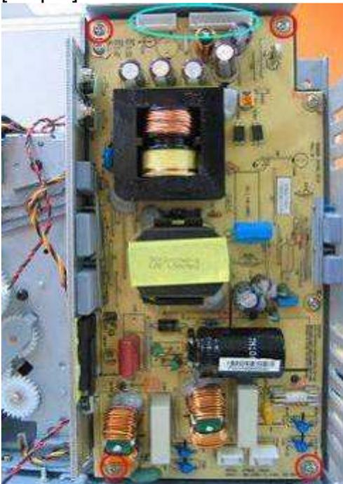
[Step 3] Replace the new POWER BD and assemble it in the reverse order of the disassembly procedure.
