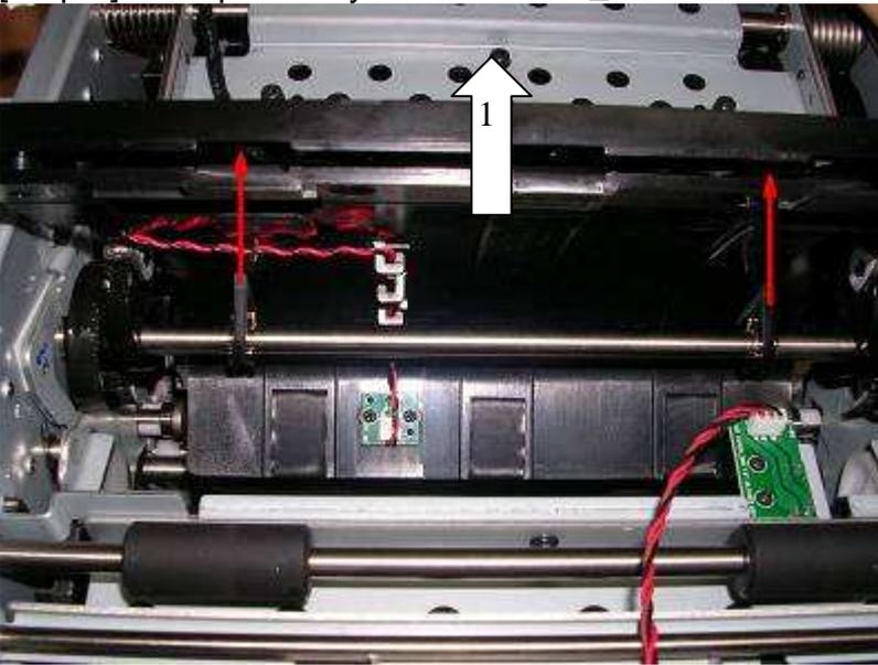
[Step 5] Uplift the TPH linkage and then pull out the tray exit.
