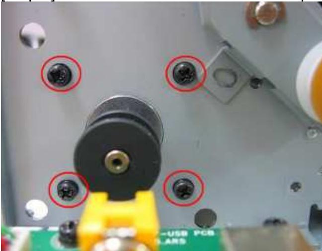
[Step 3] Replace the new capstan motor and assemble it in the reverse order of the disassembly procedure.
