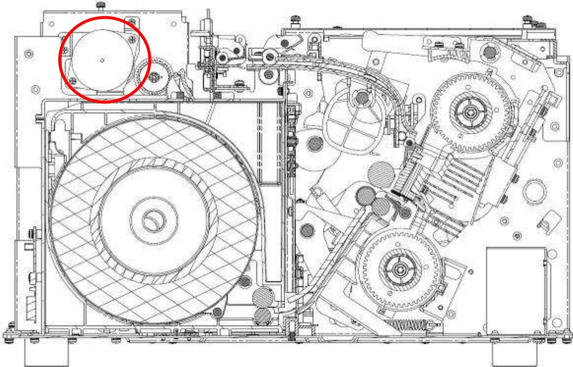
**Capstan Motor** is the most powerful motor in this printer; it controls the capstan roller through a belt and set of gears that controls the movement of the paper roll during printing process.
