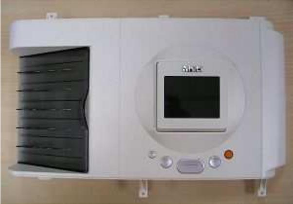
[Step 1] Remove "DOOR\_RIGHT\_A5RT", "CASE\_RIGHT\_A5RT" and "CASE\_LEFT\_A5RT", according to [Procedure No. 1](#)
