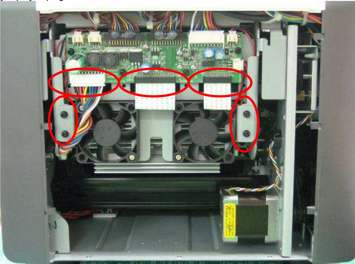
[Step 3] Remove 2 screws that hold SUB ASM TPH A5RT, and then take off SUB ASM TPH A5RT
