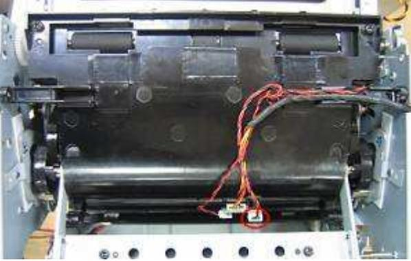
[Step 4] Pull up the tray exit from cam\_shaft.
