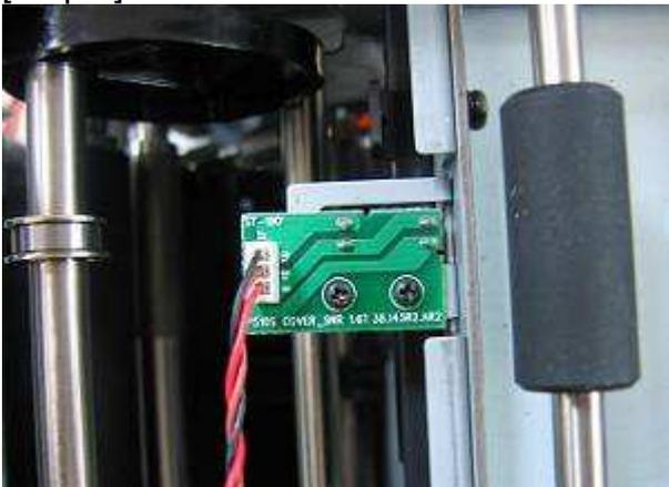
[Step 3] Replace the new cover open sensor and assemble it in the reverse order of the disassembly procedure.
