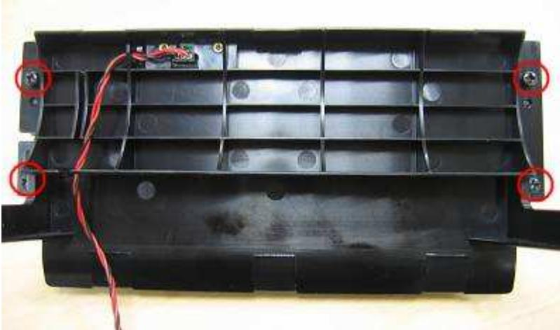
[Step 3] Remove 2 screws that hold LE Sensor, and then take it off.
