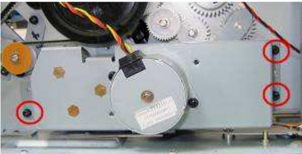
[Step 3] Replace the new ribbon take motor frame and assemble it in the reverse order of the disassembly procedure.
