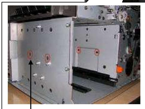
Through these 2 holes to remove 2 screws
