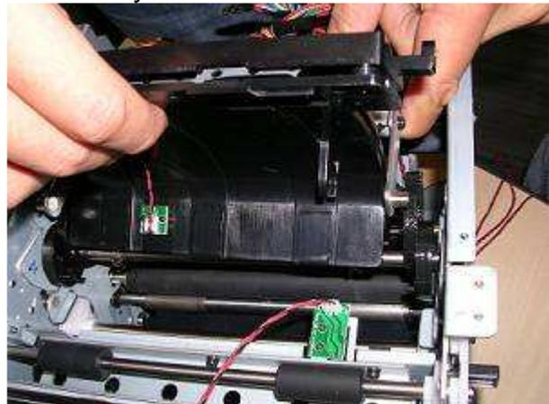
[Step 6] Replace the new Tray exit and assemble it in the reverse order of the disassembly procedure.
