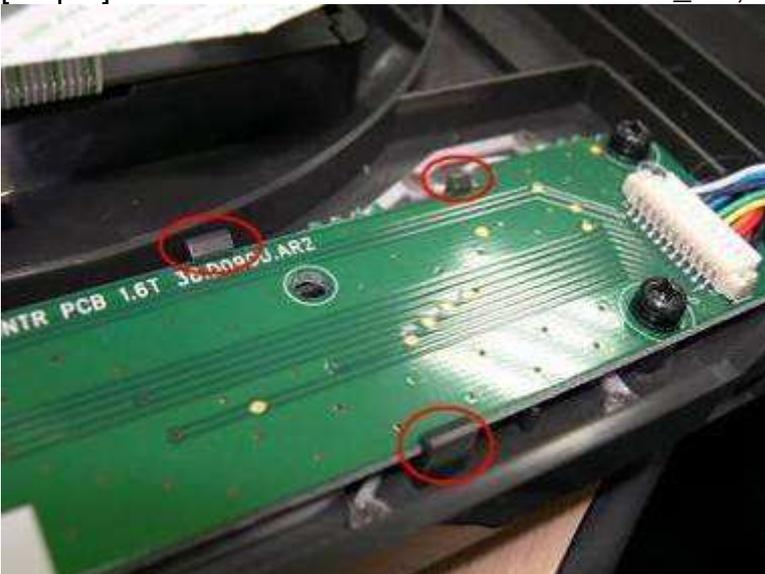
[Step 4] Replace the new BUTTON\_BD and assemble it in the reverse order of the disassembly procedure.
