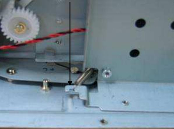
[Step 4] Remove 2 screws that hold paper box sensor, and then take it off.
