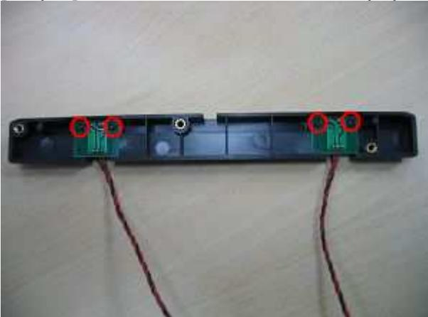
[Step 3] Replace the new paper type sensor and assemble it in the reverse order of the disassembly procedure.
