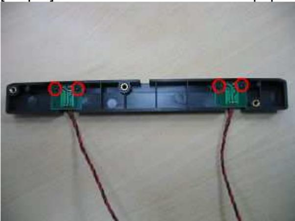
[Step 3] Replace the new paper out sensor and assemble it in the reverse order of the disassembly procedure.
