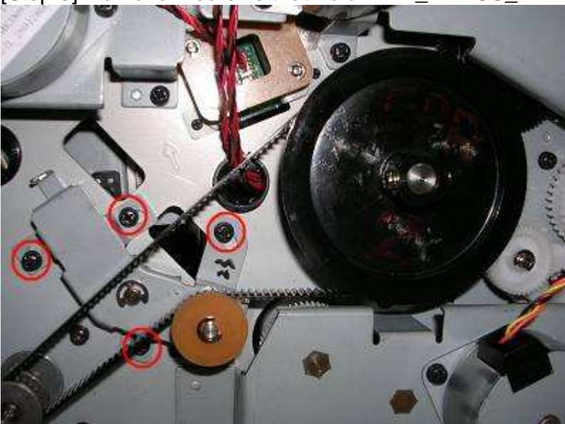
[Step 4] Remove 1 screw that hold gear\_capstan
