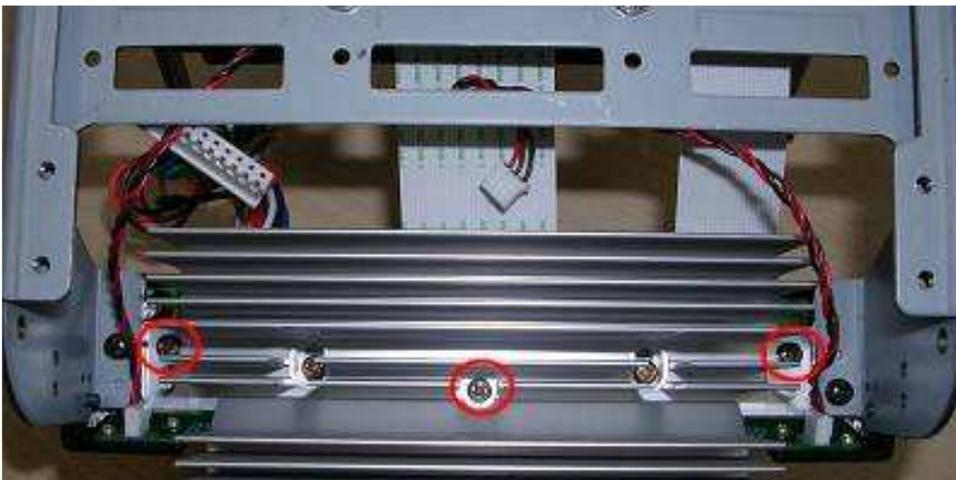
[Step 5] Replace the new TPH ASSY and assemble it in the reverse order of the disassembly procedure.
