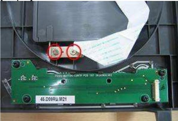
[Step 3] Reversed CASE\_TOP\_A5RT, remove 2 screws, and then take off the LCD panel frame.
