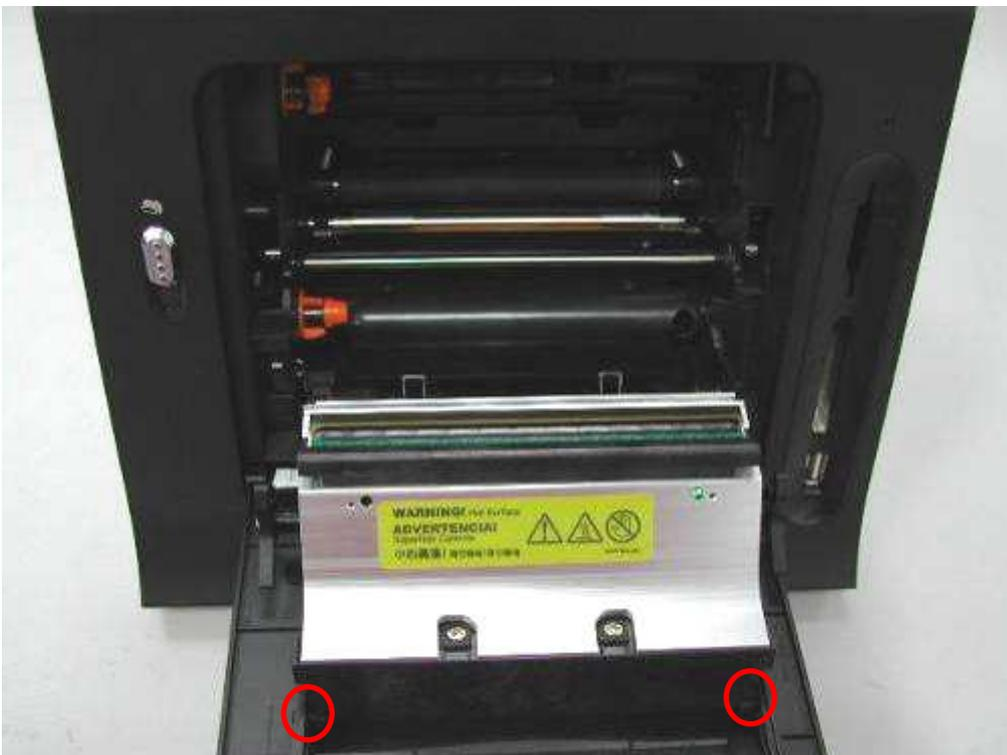
Unscrew 2 screws and unplug 7 connectors from TPH board
