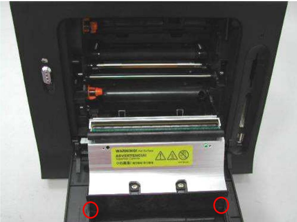
Separate case front from case back with chassis (there are two wedges in the bottom of the case front, have to unlock them firstly)
