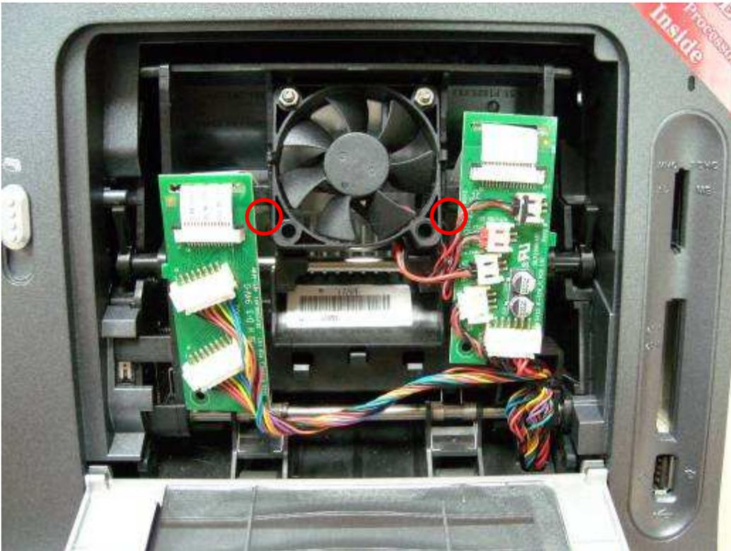
Plug 2 flat cables and screw 2 screws on TPH BD
